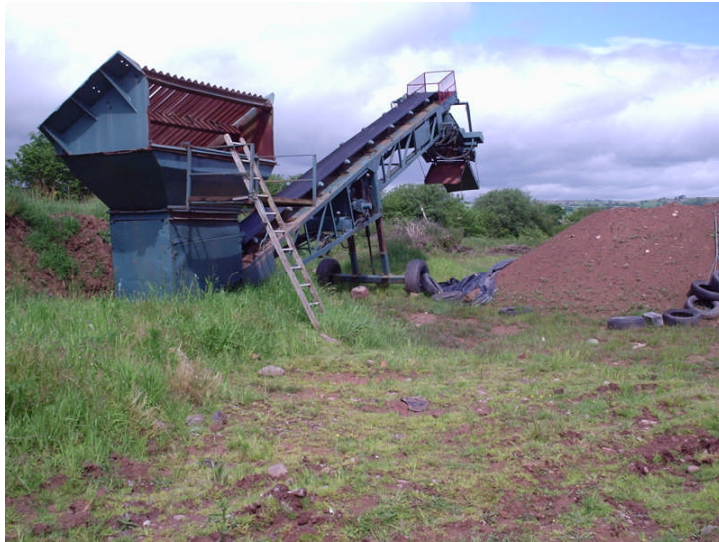
Photograph WP/3.1 Mobile Screen
